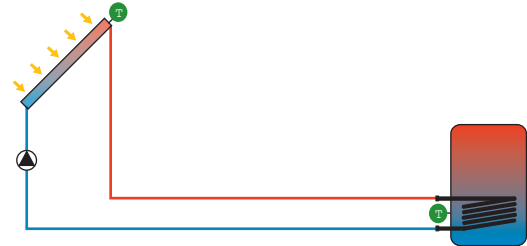
Internal heat exchanger, intelligent pump control
